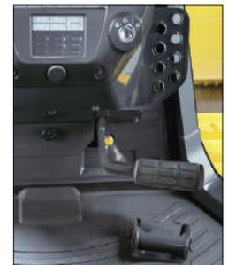
**Decelerator mode:** The pedal modulates engine rpms and vehicle travel speed. It can be used for all applications.
